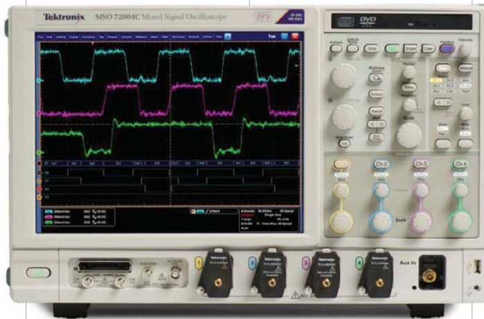
Most high-performance real-time digital scopes gain bandwidth when they interleave pairs of channels' ADCs and capture memory to double the sampling rate. The units in the 70000C series, such as this 20-GHz-bandwidth MSO72004C, in contrast, gain time resolution and SNR (signal-to-noise ratio).
