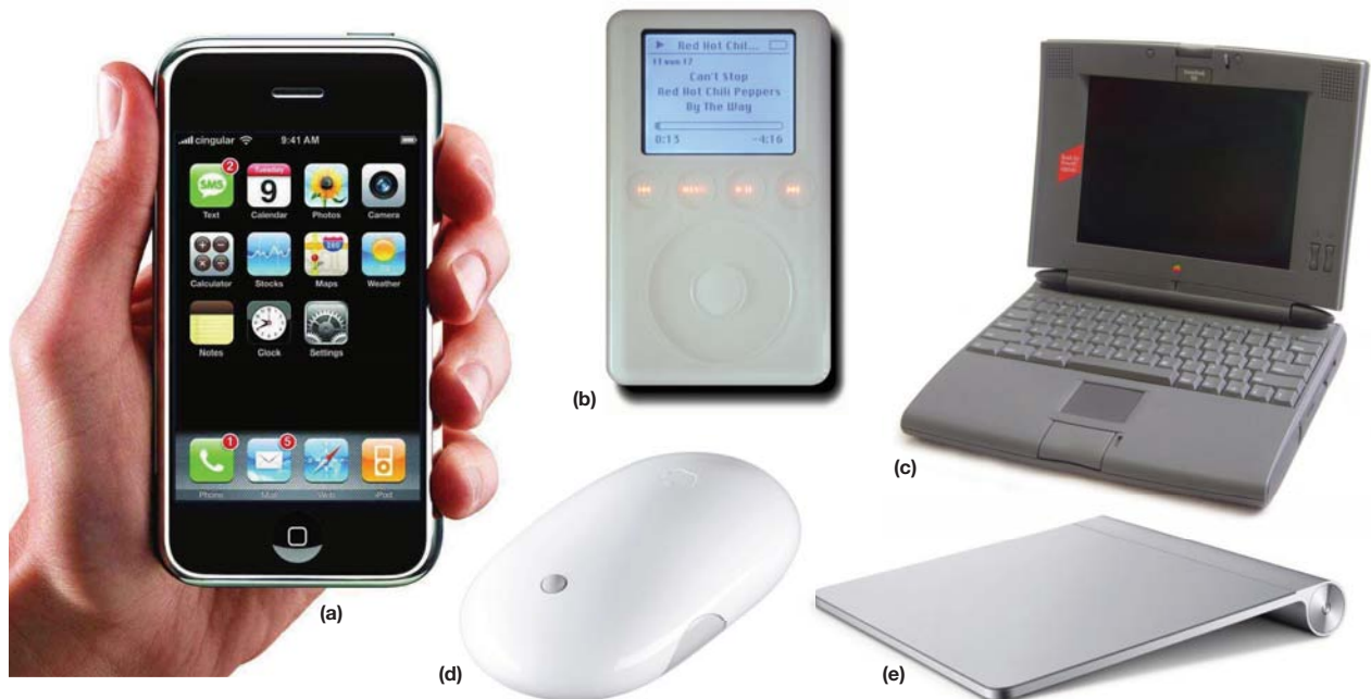
Figure 1 Apple didn't really invent multitouch, as the company claimed when it unveiled the first-generation iPhone (a) in early 2007, but it and its successors broadened public awareness of the technology. The touch wheel first appeared in the April 2003 third-generation iPod Classic (b), in which it replaced its predecessors' buttons. Apple's first laptop with an integrated track pad, replacing precursors' trackballs, was the May 1994 PowerBook 500 Series (c). The company brought capacitive touch to input devices with the August 2005 Mighty Mouse (d), and Apple began just a few months ago selling the Magic Trackpad (e), which could potentially replace the mouse.
